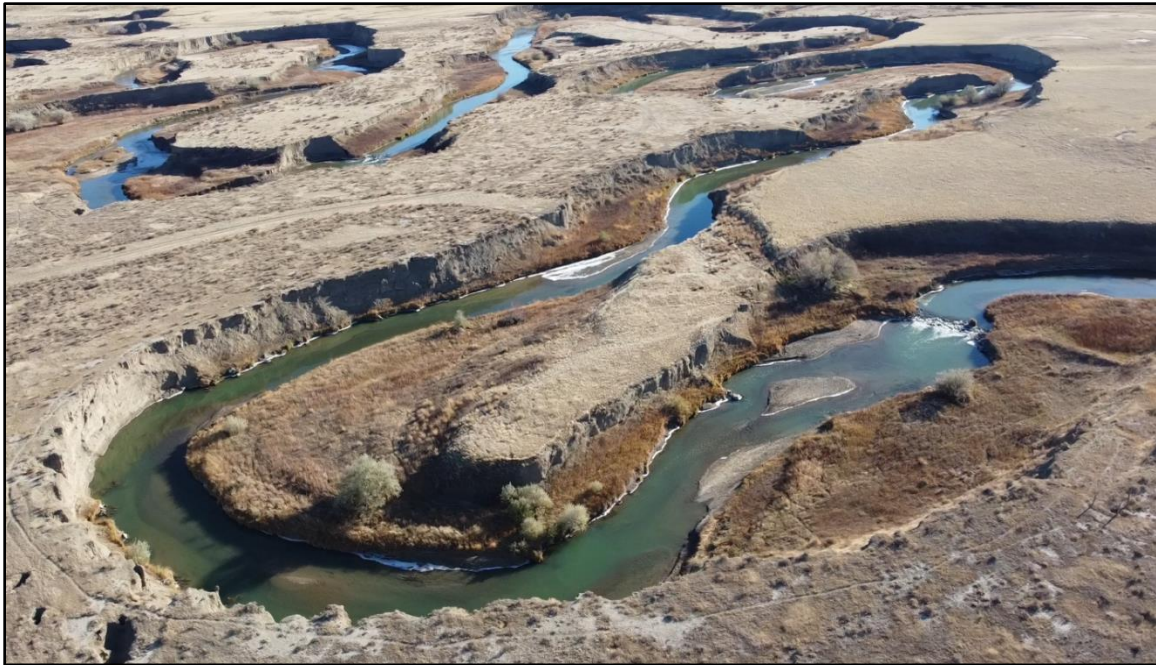
Photo 2-8. Fall 2021 drone flight clip showing deep incision along Muddy Creek (~RM 5).
