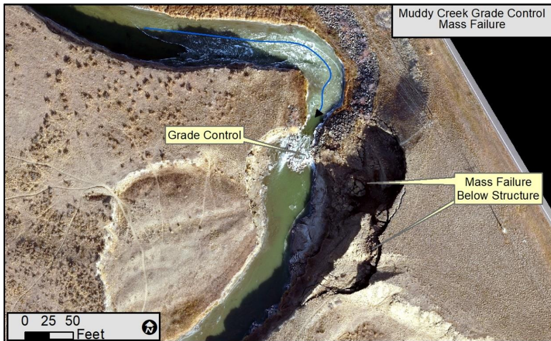
Photo 6-7. November 2021 drone image of hillslope destabilization below lowermost grade control sill, Muddy Creek RM 3.1.
