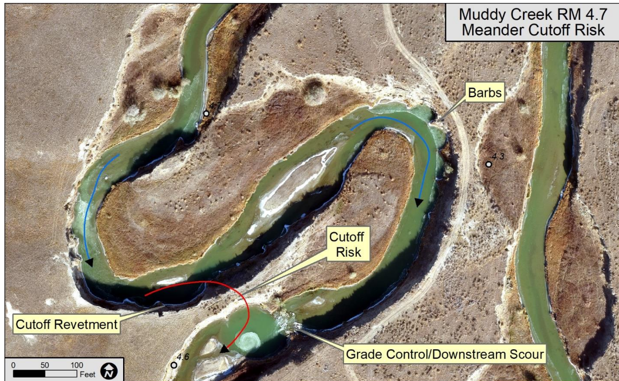
Figure 6-4. Muddy Creek meander cutoff risk, RM 4.7; note scour hole-driven bank erosion on downstream limb of meander below grade control.
