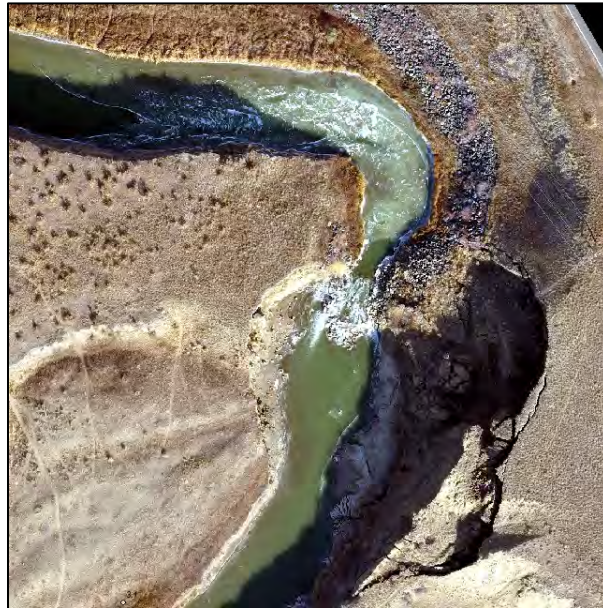
Photo 2, November 2, 2021. Drone image of hillslope destabilization below grade control, Muddy Creek (flow direction is top to bottom).
