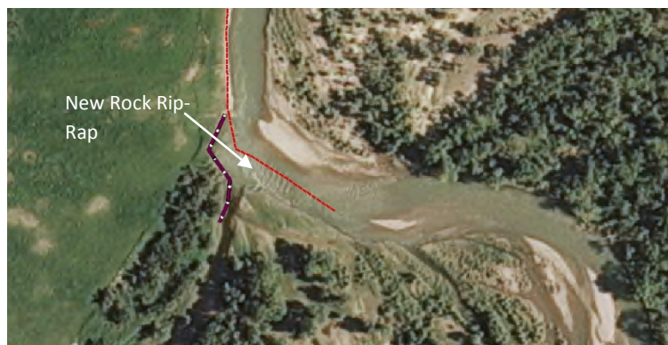
The red line depicts the 1995 bank overlain on a 2011 aerial photo. The purple line is where rock rip-rap could be placed to prevent further bank erosion and potential flanking of downstream rip-rap.
