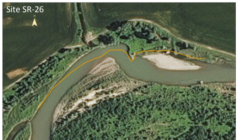
The orange line depicts the 1995 bank. Over the last 18 years, the river has eroded 50 feet into the bank.
