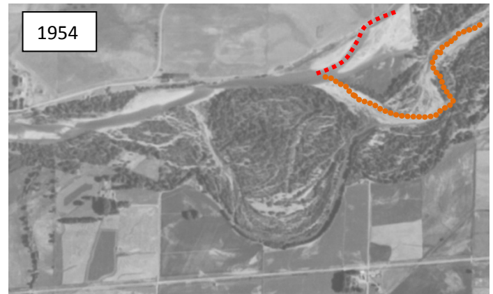
1954 Aerial Photo showing the new river channel (red dashed line) where a major avulsion occurred across a field. The 1946 channel (orange dashed line) became a secondary channel. The avulsion may have occurred during either the 1948 or 1953 flood.
