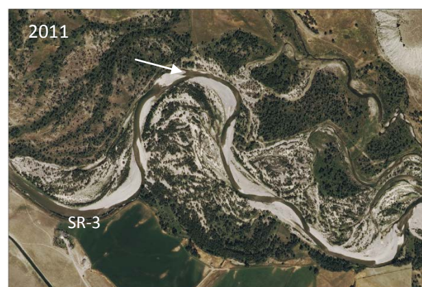
Downstream from Site SR-3. White arrow (point of reference) on the 1946 and 2011 aerial photography shows the rapid channel migration over the last 65 years.
