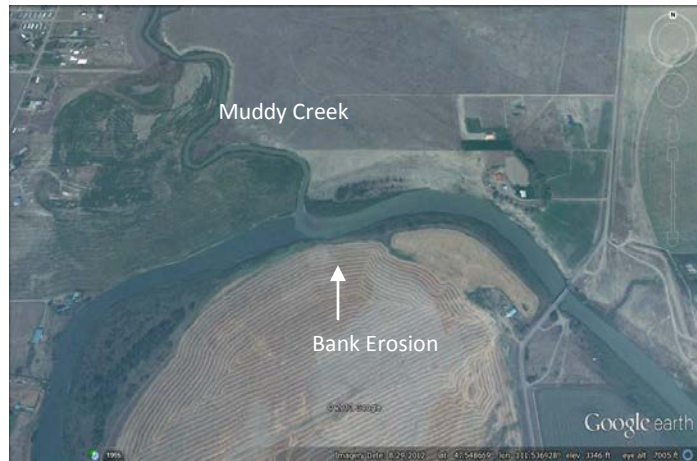
2012 aerial photo showing the Muddy Creek current directly impacting the south bank of the Sun River.
